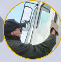
Long, large-diameter hand rails make mounting and dismounting through rear door easier and safer.
