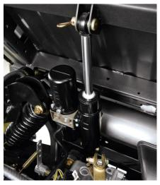
Note: T-Series are single-cylinder electromechanical; HPX is dual-cylinder hydraulic
