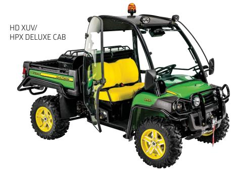
For protection from Mother Nature's worst, order a Deluxe Cab. Deluxe Cabs are certified to SAE\*1, ANSI\*1 and OSHA\*1 standards for rollover and falling object protection. Includes cab frame, glass windshield with wiper, rear window, and heavy-duty glass doors.
